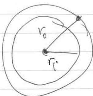
$$\text{Area(Washer)} = \pi r_o^2 - \pi r_i^2 = \pi(r_o^2 - r_i^2)$$
