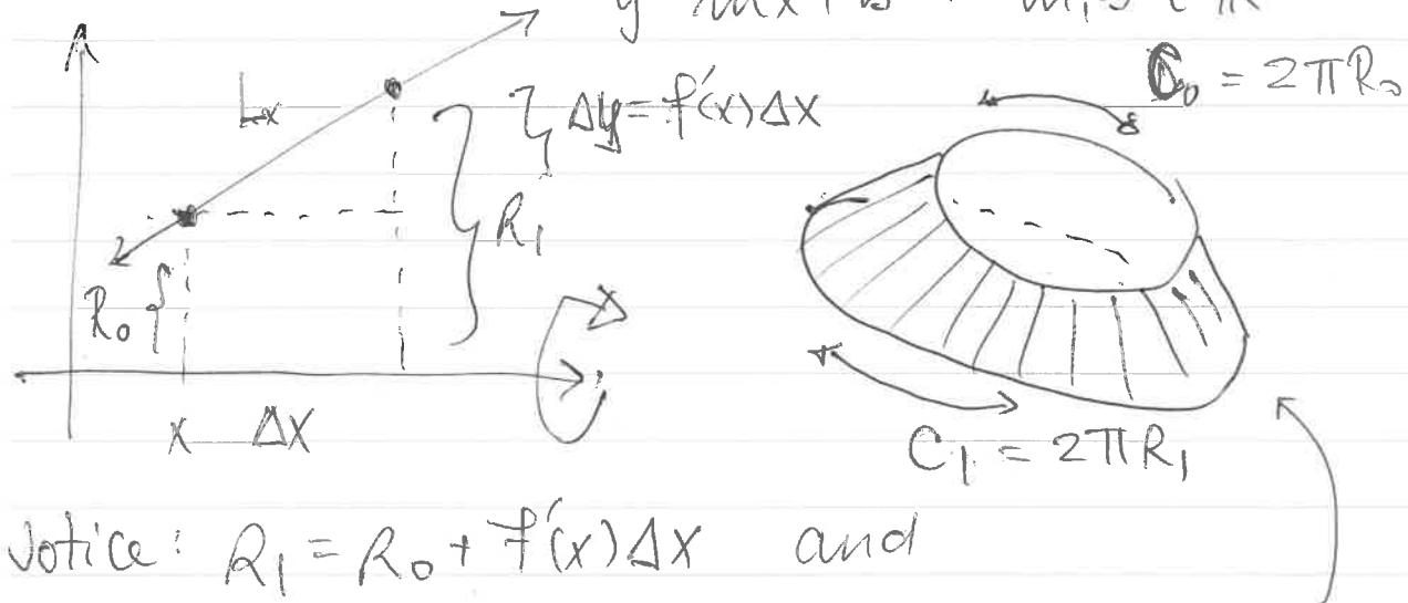
$$\text{Notice: } R_1 = R_0 + f'(x) \Delta x \quad \text{and}$$
