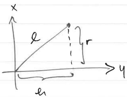
$$y = \frac{r}{h}x \Rightarrow \frac{dy}{dx} = \frac{r}{h} \Rightarrow \left(\frac{dy}{dx}\right)^2 = \left(\frac{r}{h}\right)^2$$
